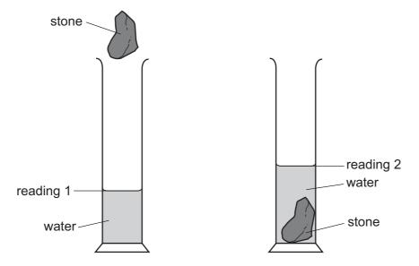
How should the student calculate the density of the stone?
