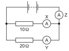
Which ammeter has the largest reading?
